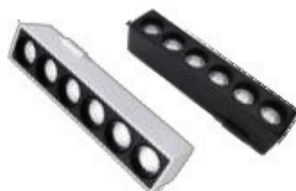
TP-2401A-C2-6 Wattage 6W CCT OSRAM 3000K /4000K /6000K CRI >90 Protectionlevel IP20 Materiel die-cast A luminum Dimension L 120*W 24*H 26 mm Track used Ultra-thin track
